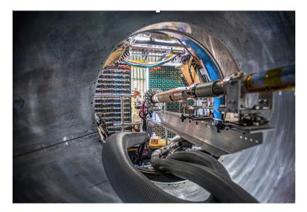
Figure 91: A view of the installed forward EMCAL, with the HCAL behind, left and right of the beam pipe.
