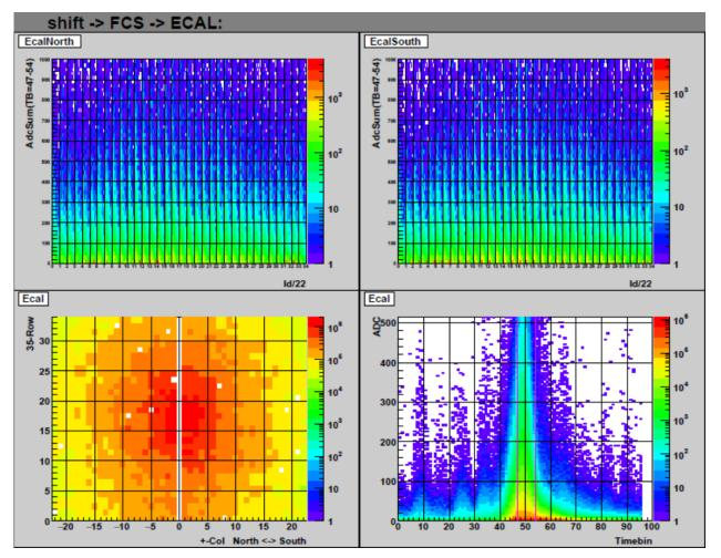
FCS EMCAL plots from online monitoring during Run-21. Bottom left: distribution of hits across all the EMCAL modules. Bottom right: energy deposition as a function of time bin in the electronics readout. Top: Energy deposition vs module ID.
