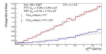
Figure 41: The expected charge mis-identification rate as a function of particle  $p_T$  in the pseudorapidity region  $2.5 < \eta < 4$  with the STAR forward upgrade. The results in blue correspond to full tracking system including both sTGC and silicon detectors and the red ones include sTGC only.
