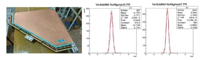
Figure 94: Left: a photograph of a pentagon-shaped sTGC module. Middle and right: residual distributions between the measured and projected positions of the  $60 \times 60$  cm<sup>2</sup> sTGC prototype in the x and y directions, respectively, from cosmic ray testing.
