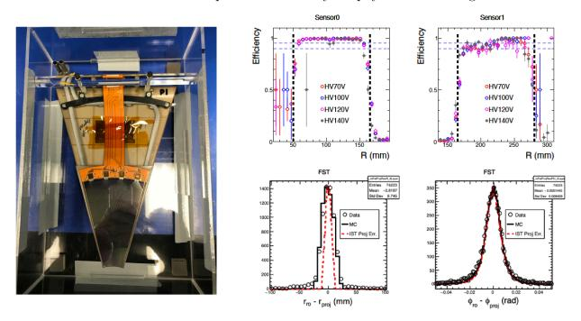
**Figure 93:** Left: a photograph of a FST detector module in the storage box with the Silicon sensor in the inner section facing up. Right: measured FST detector module performance from cosmic ray testing. Shown on the top are the efficiencies for the inner (left) and outer sensor (right) respectively. Shown in the bottom are the residual distributions between the measured and projected positions in the radial and azimuthal directions, respectively.
